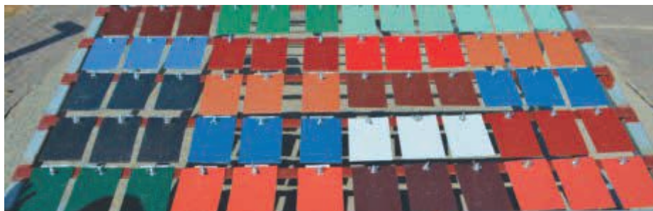
MRM corrosion site at Mariakani, Mombasa
