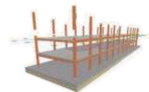
Step 5: Repeat steps 1 to 4 for the upper floors & lay concrete on floors below
