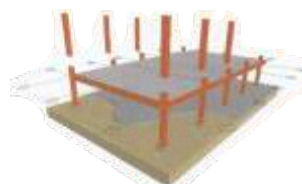
Step 4: Fixing of upper floor columns
